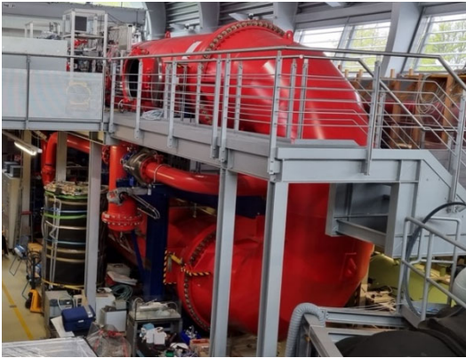
Figure 1 Left: The Variable Density Turbulence Tunnel (VDTT) at the Max Planck Institute for Dynamics and Self-Organization. Right: The ratio between the energy spectrum of the ensemble averaged velocity signal of N_T consecutive repetitions of the same experiment to the energy spectrum of one full experiment.
